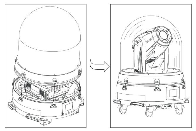
5. Finally, please cover the Dome on the fixture, and lock the 6 fast locks tightly.
