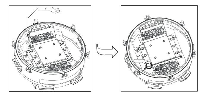
Secondly, please loosen the Thumb screws and take out the Fast Lock Wrench, then use it to loosen the 6 Quick Lock screws as the arrow direction, lift the Main Support Horizontal Plate from the base;
