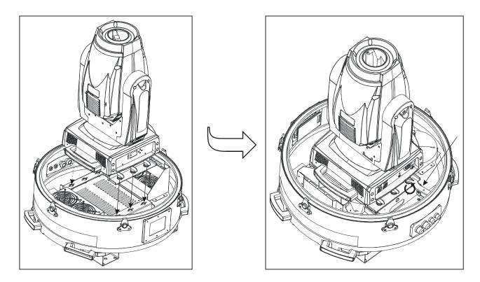
4. Then use the Fast Lock Wrench locked the 6 Quick Lock screws;
