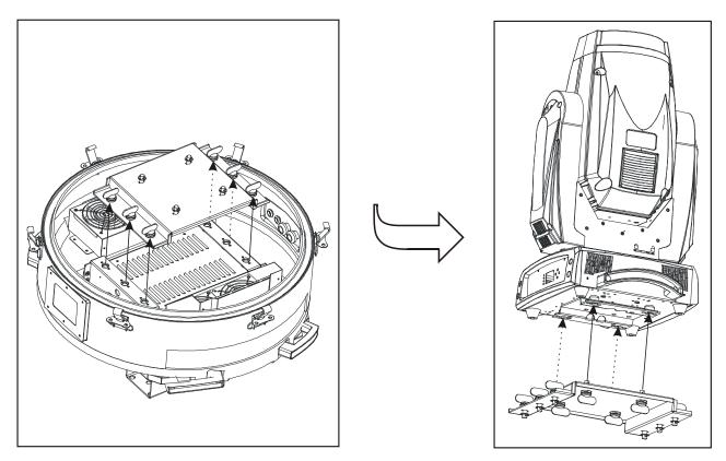
3. Now, please lock the unit on the Main Support Horizontal Plate, make sure the horizontal plate is tightly locked on the Omega clamps of the unit base;
