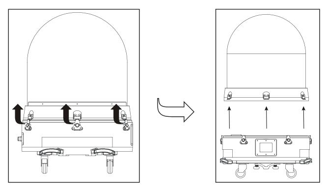
1. At first, you should loosen the 6 fast locks as the arrow direction, remove the Dome and place it in a safety location;
