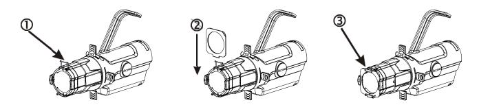
At first, please push the Lock Cap button by hand as the arrow, and move away the Lock as the arrow, then insert the color gel splint into the inside slot from topside, and fasten the lock.
