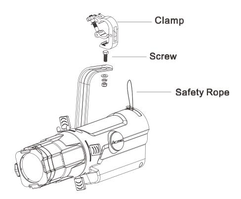
Screw the clamp to the bracket via the screw and nut. Pull the safety-rope through the fixture and over the trussing system or a safe fixation spot.
