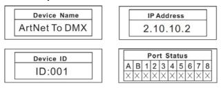
There are 4 different status (as pictures show) you can check when you power on your unit. You can switchover them by UP/DOWN button. All of the options can be changed in the main menu. In the port status, A/B means the DMX IN A/B; the 1-8 refers to the DMX output 1-8. In the status, "x" means this port is at
