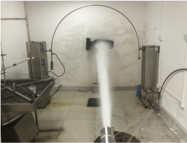
Photo 5 In the waterproof test
