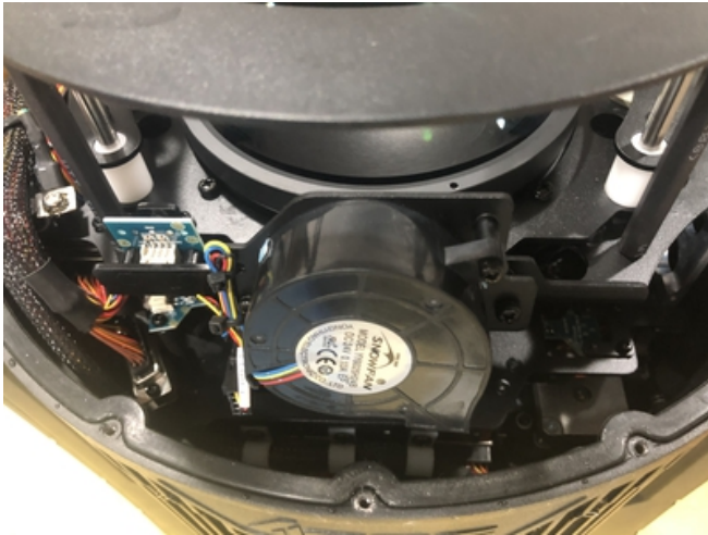
Photo 7. After the dust-proof test and the waterproof test, no dust and no water entry into internal.
