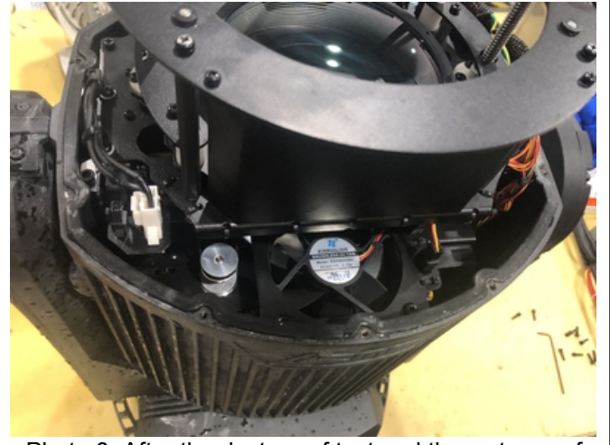
Photo 8. After the dust-proof test and the waterproof test, no dust and no water entry into internal.
