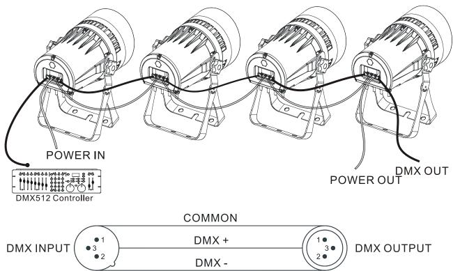
Termination reduces signal errors and to avoid signal transmission problems and interference. It is always advisable to connect a DMX terminal. (Resistance 120 ohm 1/4W)between pin2(DMX-)and pin3(DMX+) of the last fixture.
