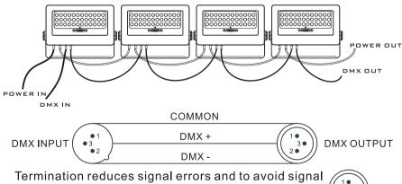
transmission problems and interference. It is always advisable to connect a DMX terminal. (Resistance 120 ohm 1/4W)between pin2(DMX-)and pin3(DMX+) of the last fixture.
