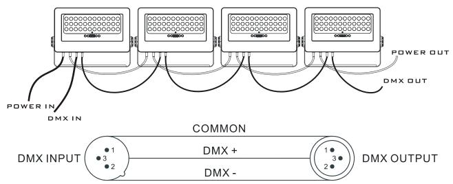
Termination reduces signal errors and to avoid signal transmission problems and interference. It is always advisable to connect a DMX terminal. (Resistance 120 ohm 1/4W)between pin2(DMX-)and
