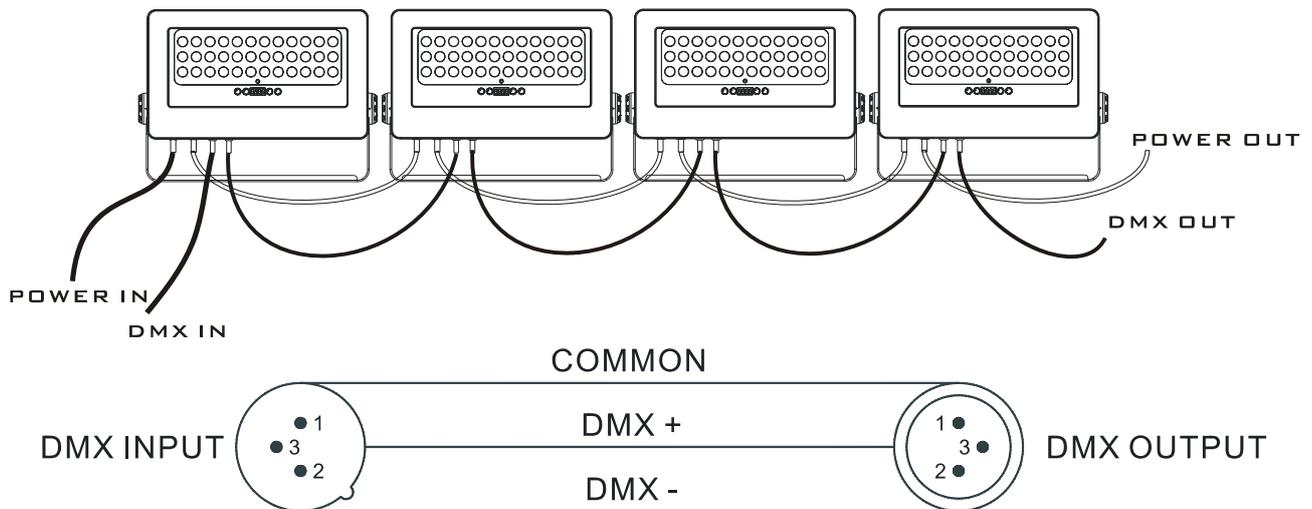
Termination reduces signal errors and to avoid signal transmission problems and interference. It is always advisable to connect a DMX terminal. (Resistance 120 ohm 1/4W) between pin2(DMX-) and pin3(DMX+) of the last fixture.
