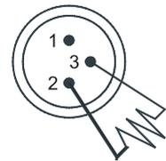
1. If you using a controller with 5 pins DMX output, you need to use a 5 to 3 pin adapter-cable.
