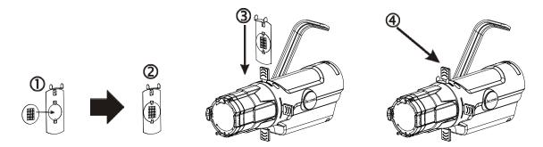
At first, put the gobo by hand as the arrow into the gobo gel splint, and insert the gobo gel splint into the slot of the unit, please turn the hand knob to left or right in order to take out gobo gel splint.
