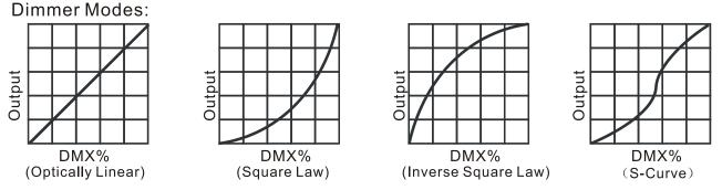
Linear: The increase in light intensity appears to be linear as DMX value is increased.
