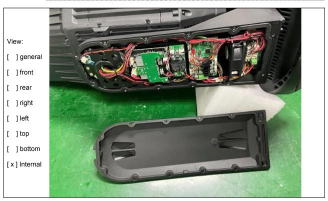
Details of: After IP66 test
