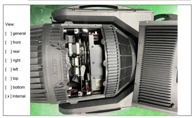
Details of: After IP66 test
