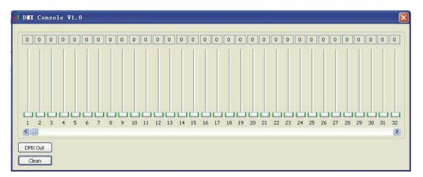
Total 512 channels DMX output, click "DMX Out" to start output, the green signal indicator LED of IU-01 blinking, push 🖾 to adjust the value.
