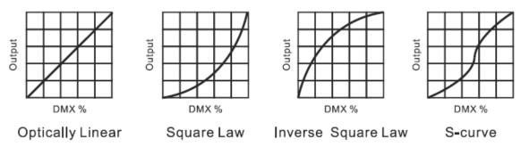
Linearity: As the DMX value increases, the increase in light intensity tends to be linear
